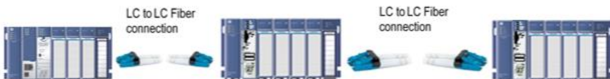
Figure 24: Interconnect using Single-Mode Fiber
