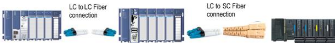
Figure 23: Interconnect using Multi-Mode Fiber
