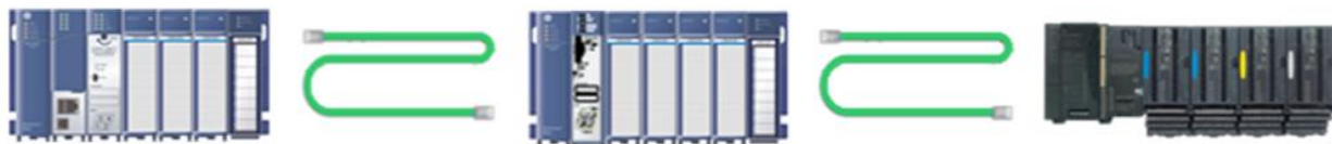
Figure 22: Interconnect using Copper Cables / RJ45 Connectors
